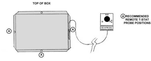
For the best operation pull excess thermostat sensing tube into the insulated space. This can be coiled.
