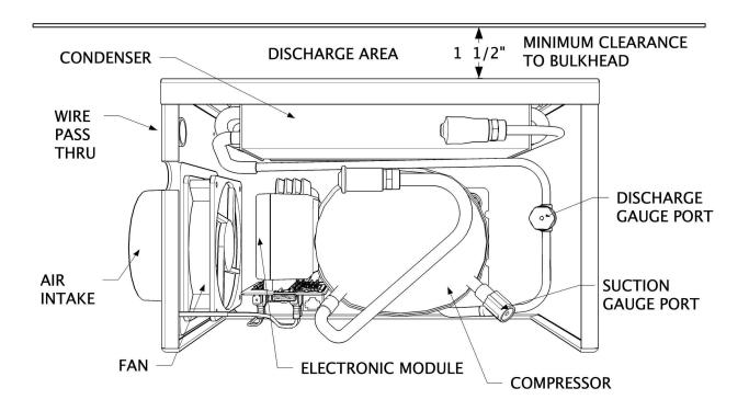
An un-ducted unit in a poorly ventilated small space will run hot, lowering the cooling capacity, increasing power consumption, and possibly causing damage by overheating the compressor.
